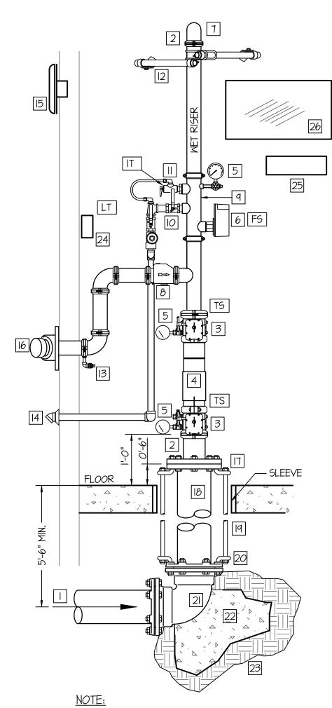
PROVIDE SLEEVES WHERE PIPING PENETRATES BUILDING AT FLOOR AND WALLS. SEAL AROUND PENETRATION WITH FLEXIBLE MASTIC AT FLOOR. PROVIDE 2" ANNULAR SPACE AROUND AND RESTRAIN FLANGE SPIGOT.
